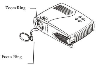
Rotate the zoom ring and focus ring until the projected image is clear and at the desired size. The projector can focus within the range of 5 feet (1.5m) to 33 feet (10m).
